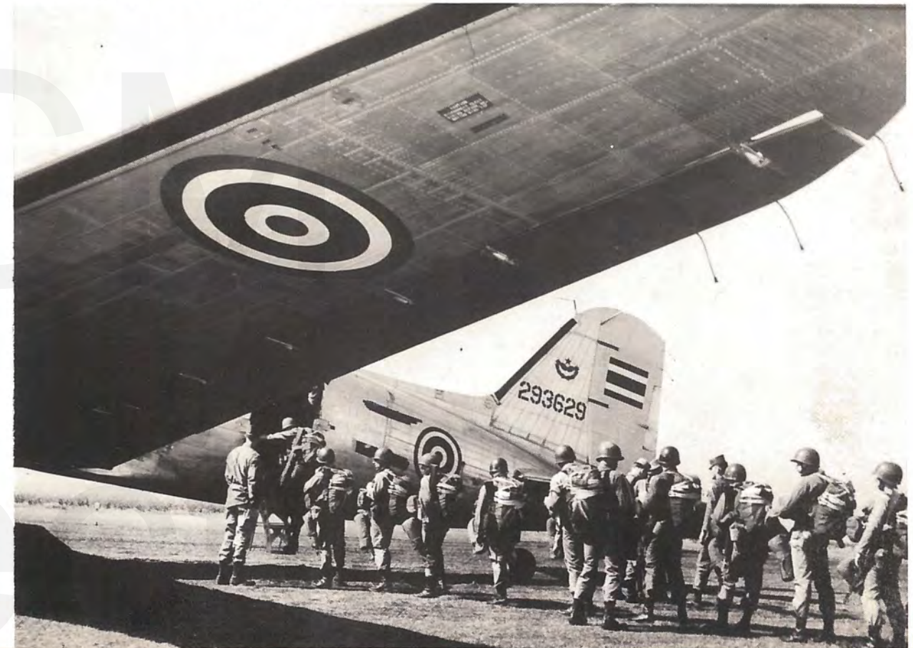
"LOAD UP": 6 Apr. 1955. Troops from the 1st Bn., 187th ARCT and 674th Abn. FA Bn., loading on a C-47 Aircraft, to jump a T-10 parachute for the first time, they had to have a different anchor line, and a five foot extension on the static line, in order to jump the T-10 from a C-47. U.S. Army Photo
