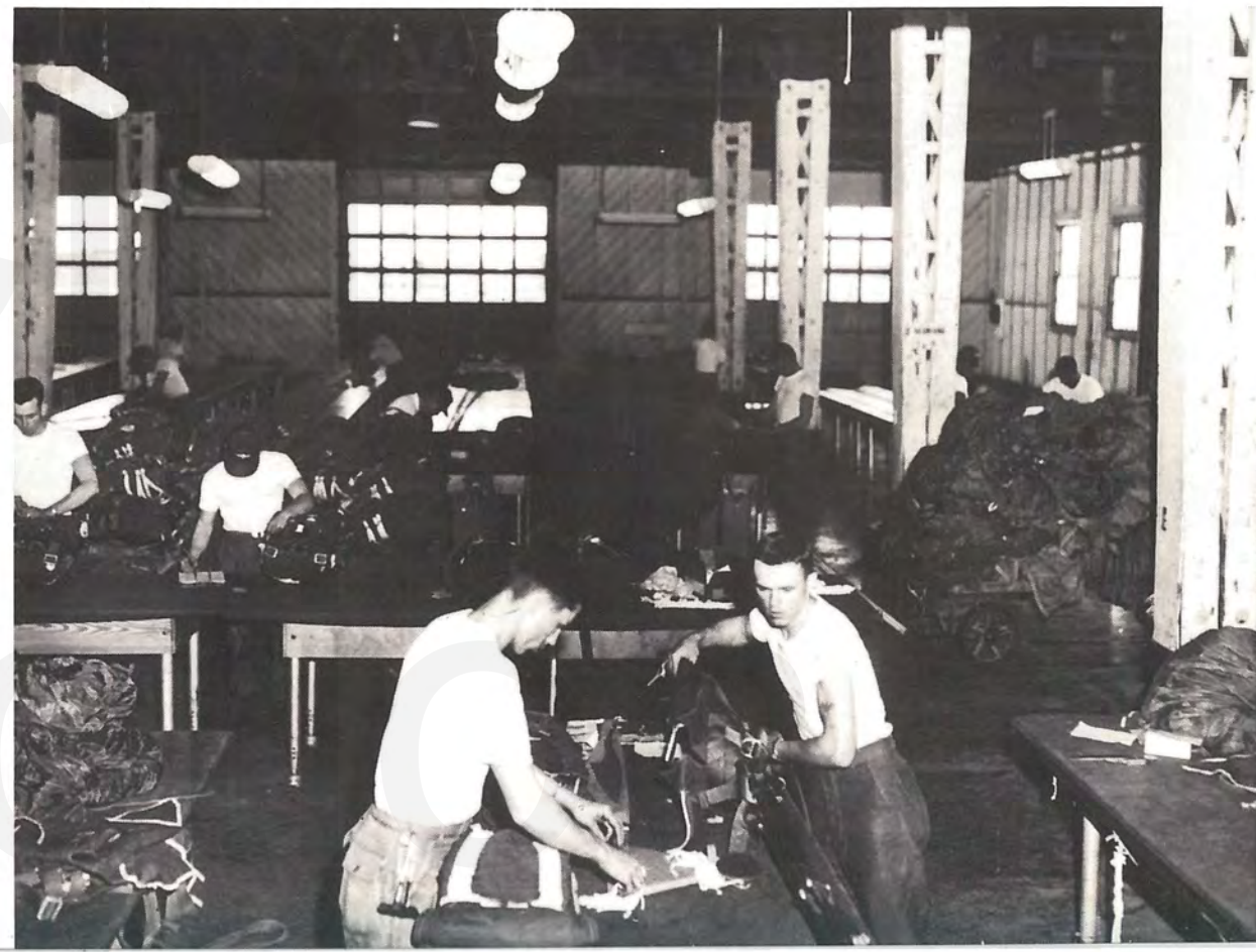
187th QM Parachute Packing Sheds. Members of the Co. are repacking and inspecting T-10 parachutes prior to their being jumped by members of the RCT.
