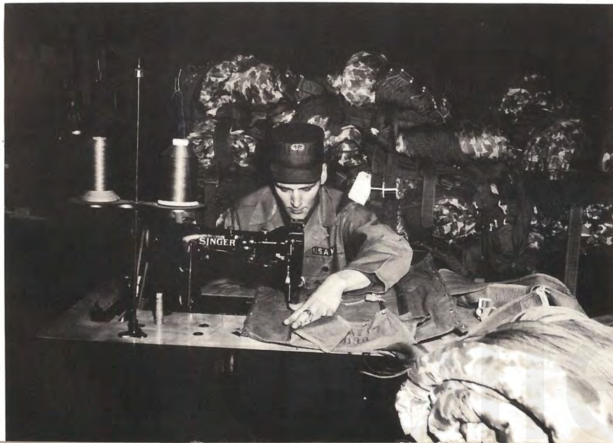
REPAIRING A CHUTE: 31 Mar. 1955. PVT Richard Miller, PM Plat., 187th ARCT here repairs a damaged side flap on a T-7 back pack assembly. U.S. Army Photo
