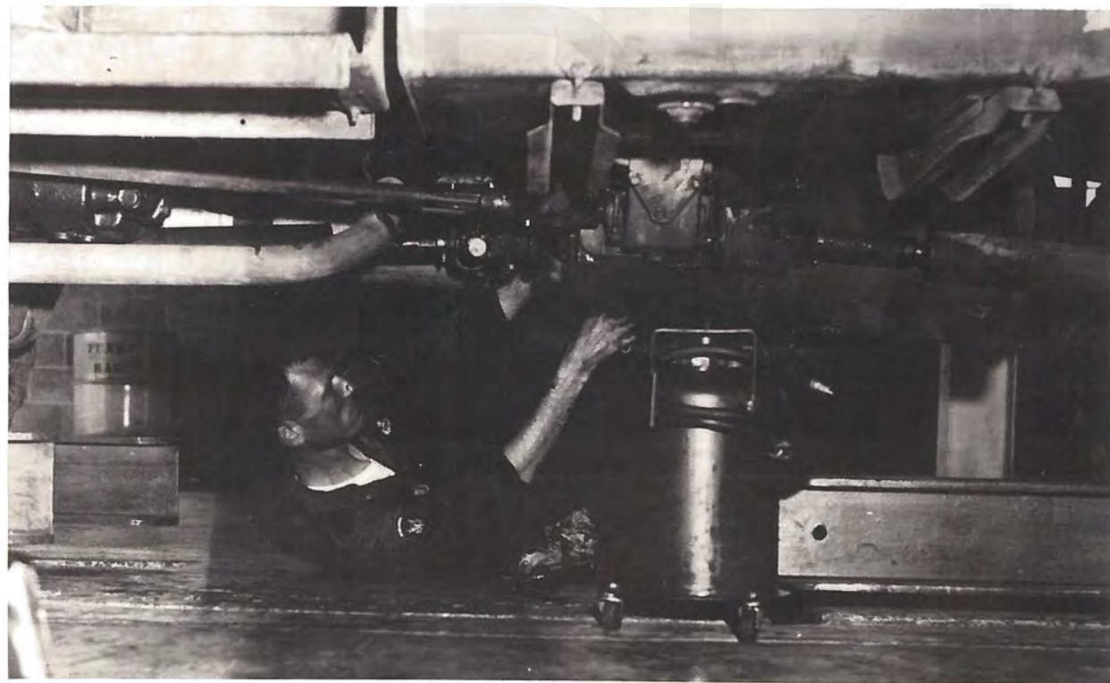
SP-2 Robert E. Jones, Svc. Btry., 674 wheel vehicle mechanic repair a drive shaft on a 674th truck.
